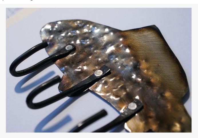
Place a hook over the hole in the fish so that they line up, and put the rivet through the holes. Flip the fish over, then take your cutters and clip the rivet so that only about 5mm (just under 1/4") protrudes from the back of the fish.
