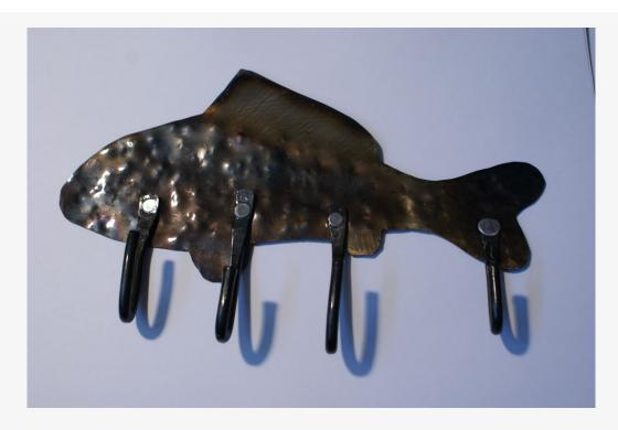
The fish is complete, but we need to protect the bare steel. Without a clear coat, it will rust in the air within days, tarnishing it forever. Clear coating should be done as soon as the piece has cooled from the flame-coloring process.
