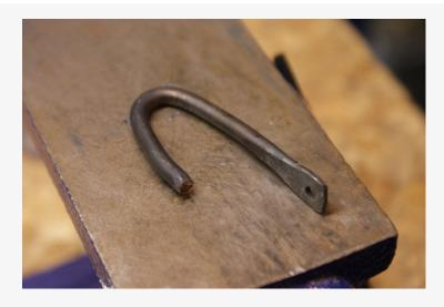
For this key holder, I decided to make my own hooks. To attach them, I wanted to hammer the end of the hook partially flat, then drill a hole through it and rivet it in place on the fish.
