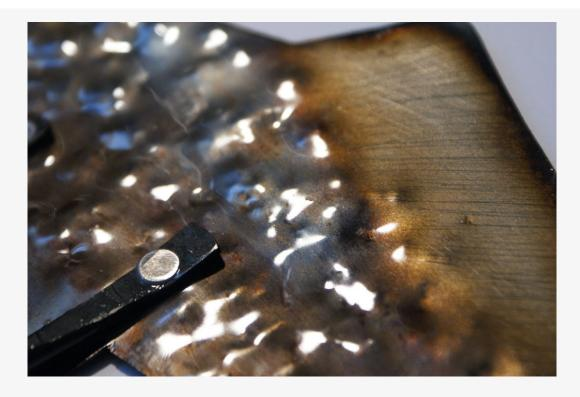
Using our 1/8" drill bit, mark with the center punch and drill four holes across the lower portion of the fish's body. I spaced mine at even intervals. Just measure your fish's length and divide by 5 to find the number you want to space them by. The fish's tail may govern where you put the last hook. Drilling the holes for the hooks now will be easier than later.
