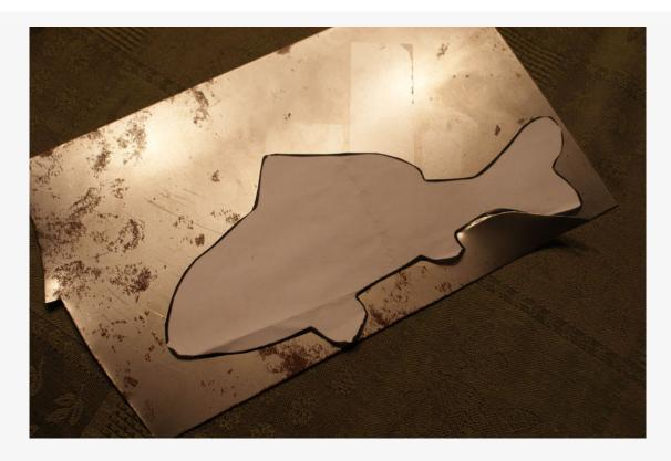
Now that our pattern is cut out, we need to tape it down so that we can score the metal around the perimeter of the shape, so we have a design on the metal to follow with our tin snips. Tape the fish cutout to the steel, and use the sharp nail or other metal implement to scratch the outline of the fish shape onto the metal. Peel off and discard the paper fish.
