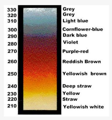
For this project, I wanted to give the fish some nice colors whilst still maintaining the reflective color and visible texture of the metal. To do this, I used a technique called flame-coloring.
