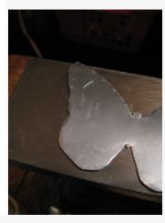
If your tin snips have tiny teeth-like textures on the jaws, then your cutout edges will end up being shiny, bumpy and very sharp. To fix this, just hammer around the edge of it on a sturdy metal surface. This will bend the metal and clean up these sharp bits that we dont want. Its best to remove them while the piece is flat.
