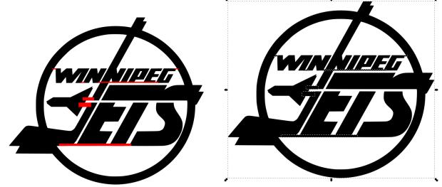
Above: The left drawing shows the rectangle bridges to join all floating parts together with red fill. The right image shows everything black and selected together.
