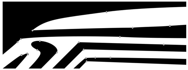
The two shapes are joined together using the Union method and after that I moved a few nodes around to make it look better and thicker using the "Edit Paths by Nodes" Tool (Shortcut: F2). If some lines are too thin they won't cut well on the Plasma Cutter
