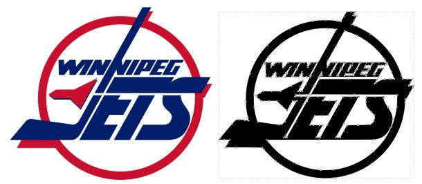
Above: Source image and the final vector design. In the future I would spend more time on this specific image to make it multi-layered and separate the original red and blue parts into 2-3 layers of metal for a 3d final layered metal design that can be welded together vs the above flat one piece design that would be cut out of one piece of metal.
